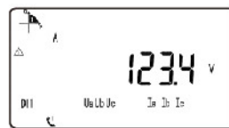
Voltage on A phase
